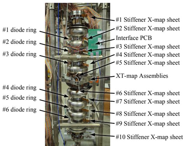
Figure 3: XT-map (1 cell) and Stiffener-X-map (10 strips) test circuits and its installation with vertical test at JLab.
