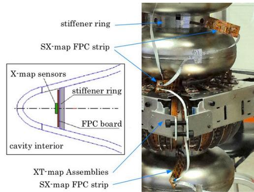
Figure 4: Stiffener-X-map FPC strips are installed under the stiffener rings.
