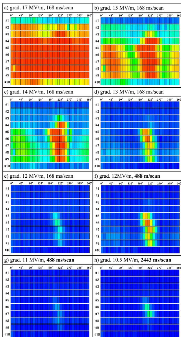
Figure 6: The screen shots of measurement results with Stiffer-X-map. For example, #6 SX-map board is installed at an iris between 5th and 6th-cell from the cavity top. And the locations of #1 and #10 are top and bottom flanges. The horizontal axis is an angle of sensor position on each iris. The signal display becomes close to red so that an output signal is strong.
