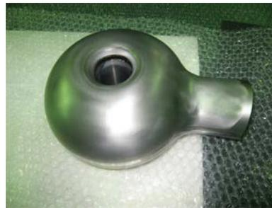
Figure 2: drift tube and stem.
