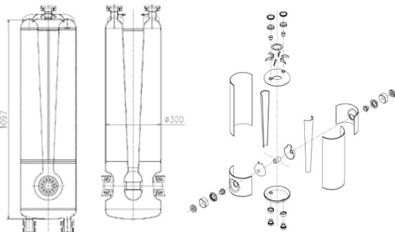
Figure 1: 73MHz prototype QWR for RIKEN.
