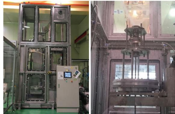
Figure 5: High pressure rinse facility.
