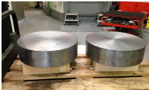
Figure 1: CBMM Large Grain ingots at Heraeus in preparation for the slicing process.
