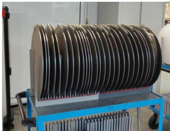
Figure 2: Large Grain ingots after slicing at Heraeus.
