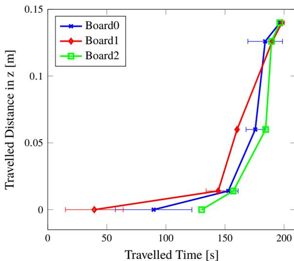
Figure 3: This figure depicts the path of the superconducting phase through the cavity. It is displayed for 3 different PCB boards. This measurement was done during a warming up above the critical temperature that was done with a heater connected to the lower beam pipe of the cavity. Every point is displayed with the  $1 - \sigma$  uncertainty.
