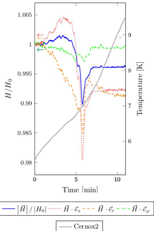
Figure 2: The left axis indicates the measured field normalized to the constant field value at the time  $t = 0$  min. The right axis denotes the temperature measured with the cernox sensors. Only the results of *Cernox 2* are plotted. *Cx2* measured the temperature at the top flange of the cavity’s beam pipe. Its position is shown in Fig. 1 as red dots.
