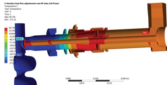
Figure 5: Thermal distribution in the coupler.
