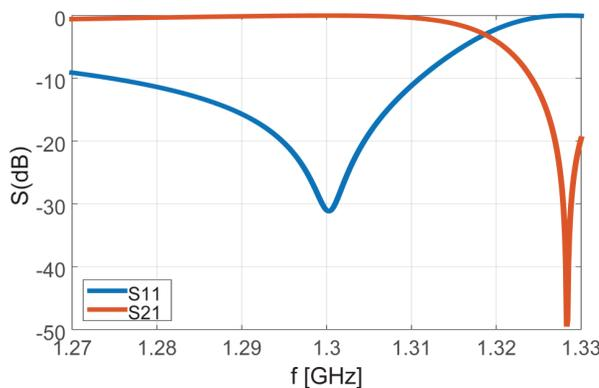
Figure 4: S parameters of the coupler.
