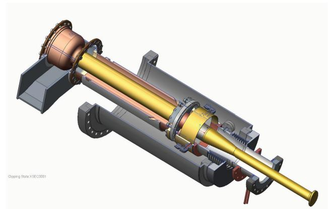
Figure 1: Cut away of the complete coupler.
