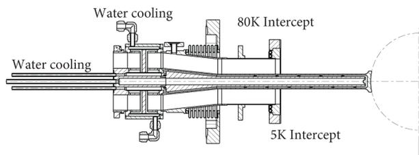
Figure 7: Cooling locations on the cold part of the coupler.
