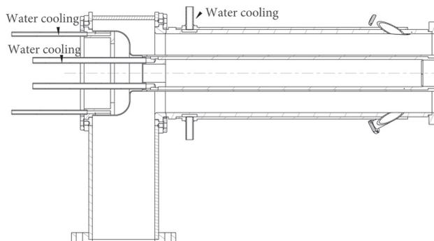
Figure 6: Cooling locations on the warm part of the coupler.
