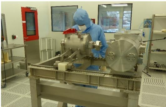
Figure 3: trial assembly in cleanroom with dummy components
