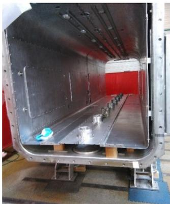
Figure 7: blank assembly of the thermal shield inside the vacuum vessel.
