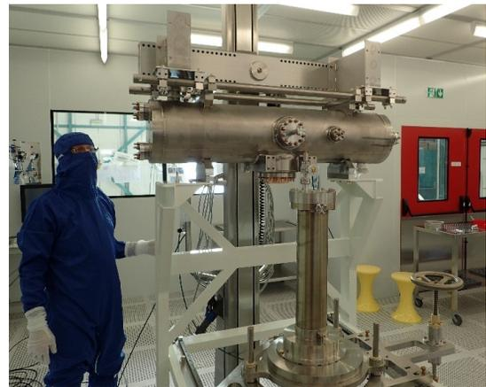
Figure 5: cavity coupler assembly in cleanroom, cavity installation onto the bench
