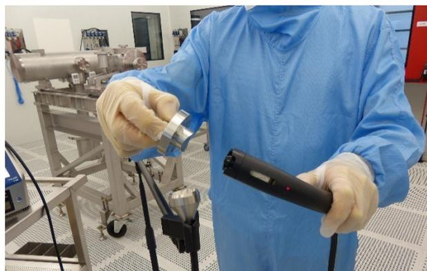
Figure 2: nitrogen blowing of a BPM button before its assembly
