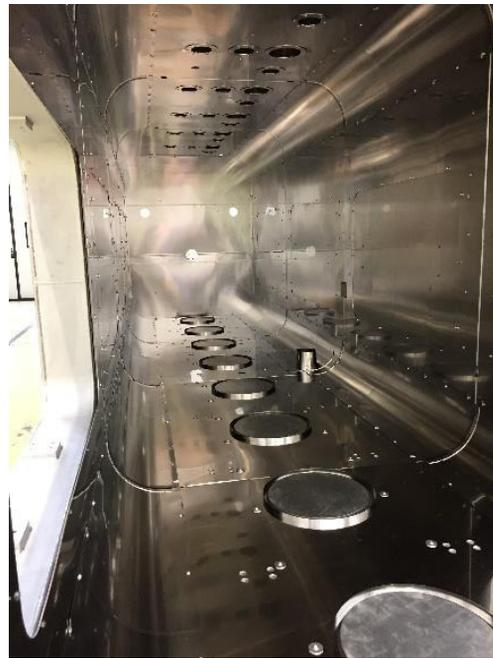
Figure 5: Magnetic shield installed in the vacuum vessel.
