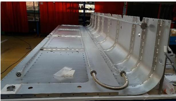
Figure 7: Partial assembly of two panels of the thermal shield.
