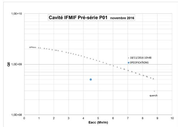
Figure 2: Vertical test results of the first manufactured HWR.
