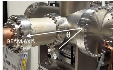
Figure 1: DSu fiber optics coupling assembly located on the PTank, with an observation angle  $\theta = 25^\circ$ .
