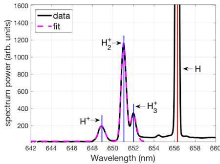
Figure 2: Typical spectrum from the DSu showing the Balmer  $\alpha$  ray and Doppler shifted rays of H,  $H_2$  and  $H_3$ . The vertical lines are positioned using Eq. (1).
