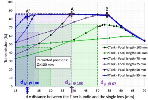
Figure 3: Light transmission calculated with APILUX.
