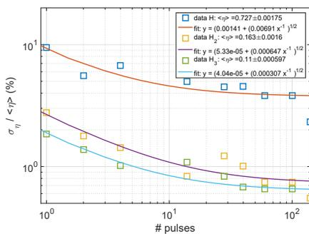
Figure 4: Statistical fluctuation of the fraction species measured with the DSu, in single shot acquisition of 3 ms exposure. The trigger delay is 3 ms. The current is 70 mA, the pulse length is 6 ms. The graph shows the standard deviations of the fractions (squares) as function of number of pulses acquired and averaged in software.
