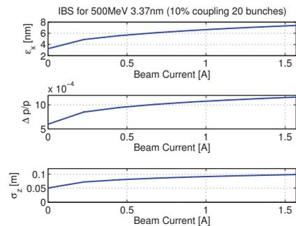
Figure 4: The ring emittance with IBS.
