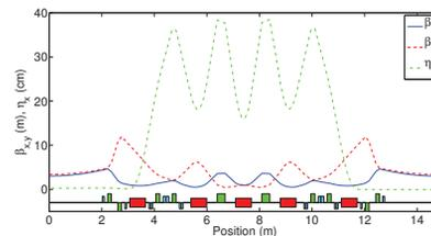
Figure 1: Ring optic functions: horizontal beta function (blue), vertical beta function (red dash), and horizontal dispersion (green dash).
