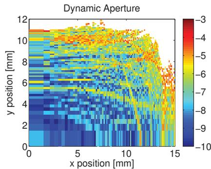
Figure 2: Dynamic aperture and diffusion rate of the ring.
