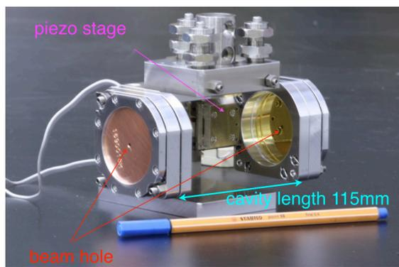
Figure 4: Cavity assembly.
