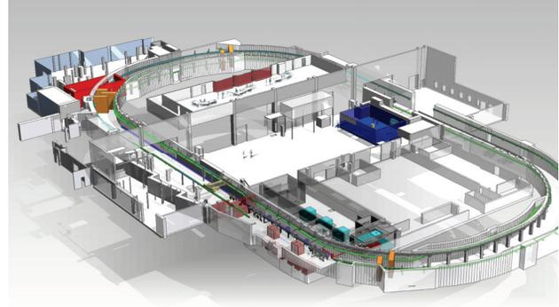
Figure 1: Overview of the SINBAD R&D facility. Only half of the available tunnel area will be used for the two initial experiments.
