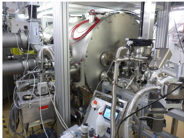
Figure 3: Gun-1 module in GunLab. In front of the module the cathode transfer system can be seen. From the left the cold box cryo supply lines are connected to the module.
