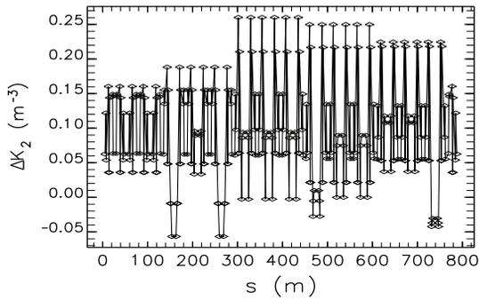
Figure 4: The sextupole strength error calculated from all the study lattices.
