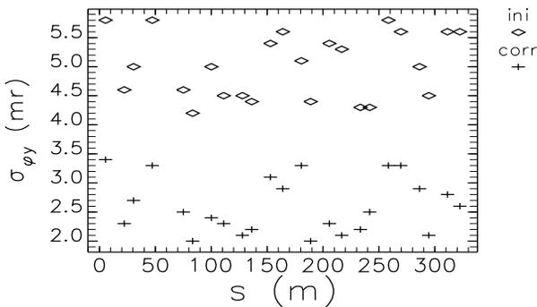
Figure 5: The vertical phase error before and after one correction. Each point corresponds to a study lattice which is perturbed by one corrector at the shown location. The bending angle is about 0.2mrad for all the correctors.
