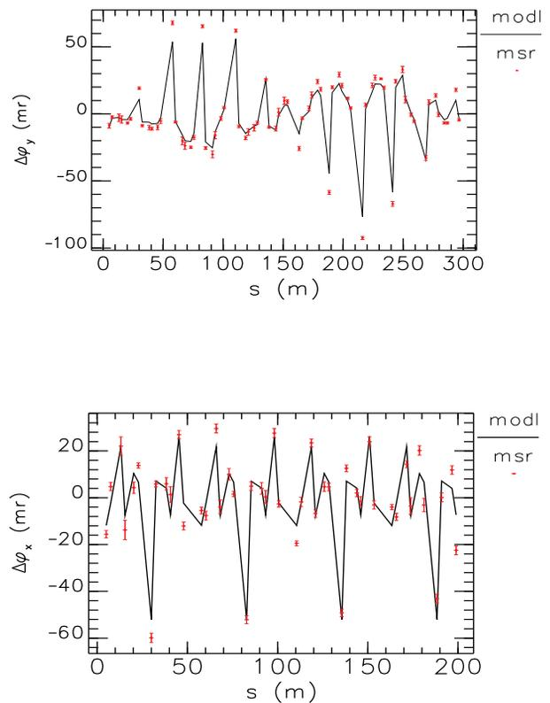
Figure 2: The measured and the calculated phase change caused by the off-centered sextupoles. Top: The corrector was changed by 0.18 mr. Bottom: The momentum offset was -0.6%. The error bar was obtained from 6 measurements. They correspond to the orbit change in Fig. 1, but only one plane is plotted. In both cases only part of the ring is shown for clear view.
