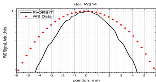
Figure 5: The horizontal profiles at MEBT WS14. The line is a PyORBIT reconstruction, and the points are WS data.
