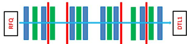
Figure 1: The SNS MEBT structure. Blue and green colors denote horizontally and vertically focusing quads, respectively, and the red signifies RF buncher locations..
