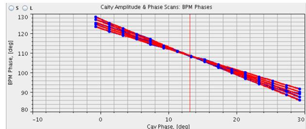
Figure 2: The results of the buncher #4 phase scans for different buncher amplitudes.
