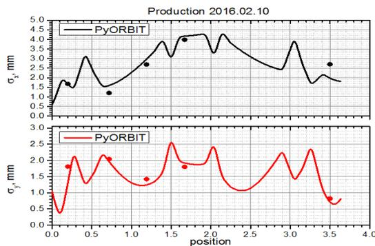
Figure 4: The horizontal (black) and vertical (red) RMS sizes of the beam in the MEBT during production on 2016.02.10. Lines are from the PyORBIT reconstruction, and points are WS data.
