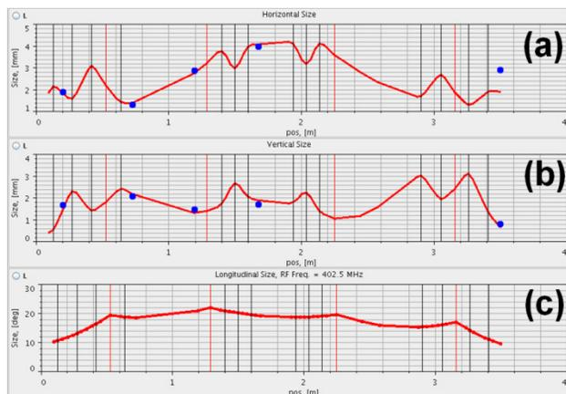
Figure 3: The RMS sizes of the bunch in the SNS MEBT. (a),(b),(c) are horizontal, vertical, and longitudinal RMS sizes, respectively. The red line is taken from the Online Model, and blue points are WS results. The vertical black lines are centers of quads, and the red ones are the RF bunchers.
