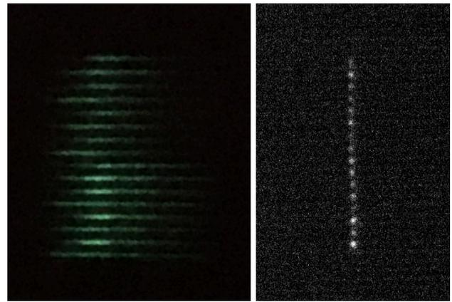
Figure 2: Streak camera images of UV laser (left) and electron beam OTR (right) showing an evenly spaced 16 bunches.
