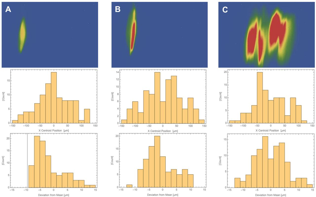
Figure 3: Spectrometer screen images and histograms of the calculated centroid position and width for a single bunch in A; 2 bunches in B; and 16 bunches in C. Energy jitter is uniformly 0.07%; energy spread is 0.04% for 1 and 2 bunches, and 0.16% for 16 bunches.
