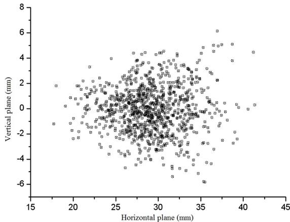
Figure 5: The beam profile at the neutron target for the case of the horizontal beam displacement at the beam monitor equal to 29 mm (2 RMS beam displacement value) in the horizontal plane.
