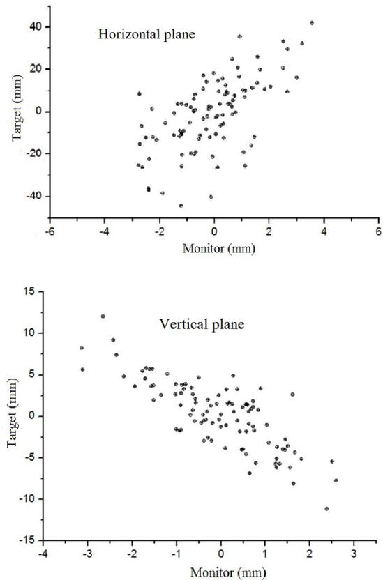
Figure 4: Correlation of the beam position at the beam position monitor and the neutron generating target.
