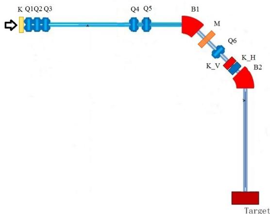
Figure 1: The layout of the NSC KIPT Neutron Source transportation channel: B1-B2 are 45 degree bending magnets, Q1-Q6 are focusing quadrupoles, K, V – K, H are scanning bending magnets, K is dipole corrector, M is beam position monitor.
