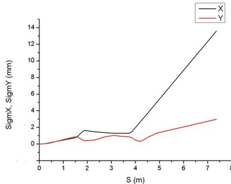
Figure 3: RMS beam position displacement along transportation channel.
