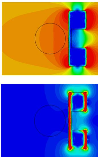
Figure 5: Simulation of the main field with a single (asymmetric) conductor: (a) 61mT at the peak of the current pulse; (b)  $\sim 800 \mu\text{T}$  at  $3 \mu\text{s}$  after the current pulse.
