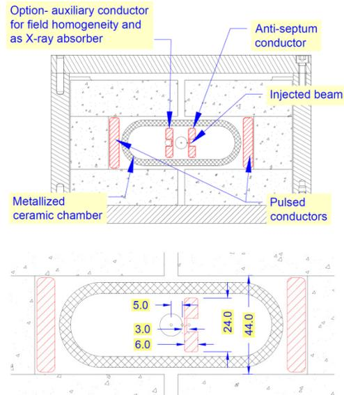
Figure 3: (a) Cross section of kicker and (b) dimension details of the anti-septum conductor.
