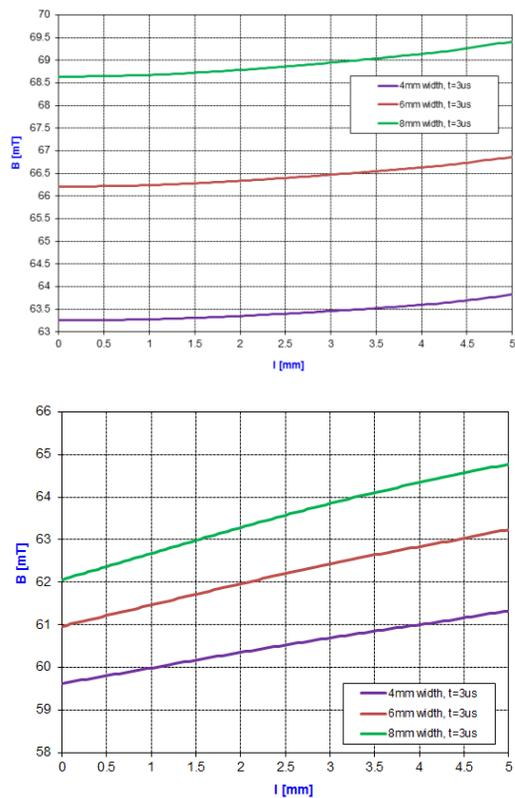
Figure 6: Main pulse homogeneity  $x=0 \text{ mm}$  to  $x=5 \text{ mm}$  for (a) dual (symmetric) conductors and (b) single (asymmetric) conductor, with conductor thickness 4, 6 and 8 mm.
