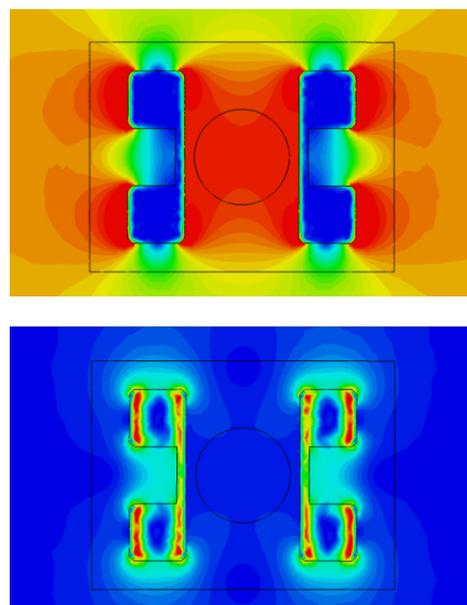
Figure 4: Simulation of the main field with symmetric conductors: (a) 66 mT at the peak of the current pulse; (b) ~800 μT at 3 μs after the current pulse.
