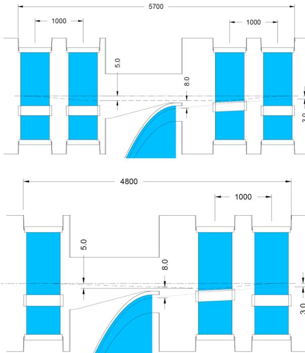
Figure 2: (a): Schematic plan view of the injection straight with a symmetric bump and the added anti-septum. (b): As for (a) but with three kickers of unequal strengths 1.6, 6.2 and 4.6 mrad.
