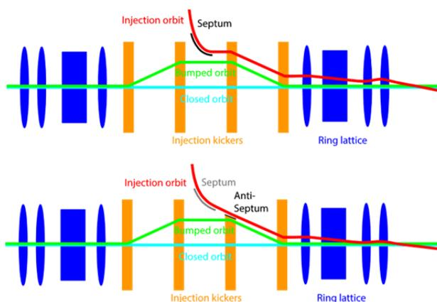
Figure 1: Schematic views of conventional top-up injection schemes with normal septum (upper) and anti-septum (lower).
