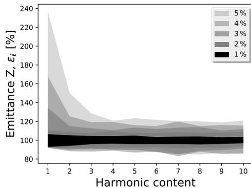
Figure 9: Predicted longitudinal emittance increase as a function of the harmonic content.
