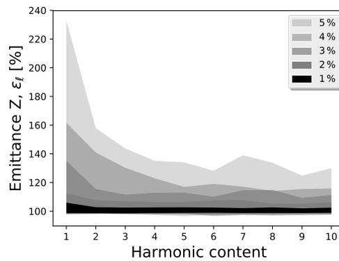
Figure 5: Simulated longitudinal emittance increase as a function of the harmonic content.
