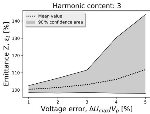
Figure 7: Predicted longitudinal emittance increase as a function of the voltage error.
