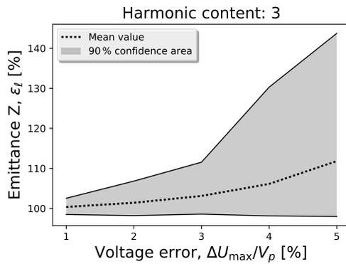
Figure 3: Simulated longitudinal emittance increase as a function of the voltage error.
