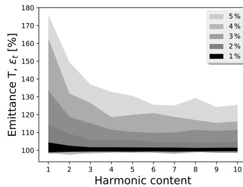
Figure 10: Predicted transverse emittance increase as a function of the harmonic content.
