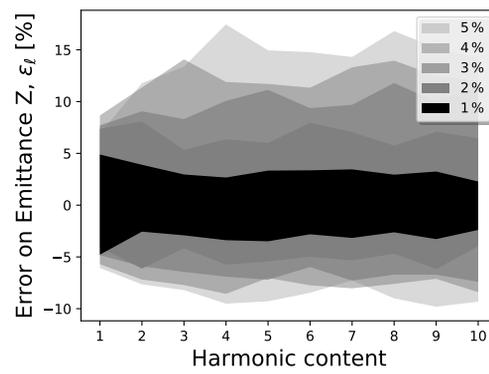
Figure 11: Errors on the predicted longitudinal emittance.
