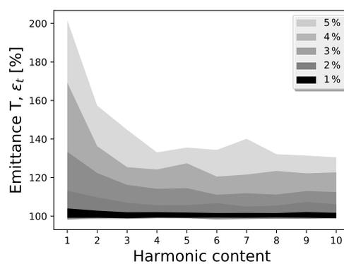
Figure 6: Simulated transverse emittance increase as a function of the harmonic content.
