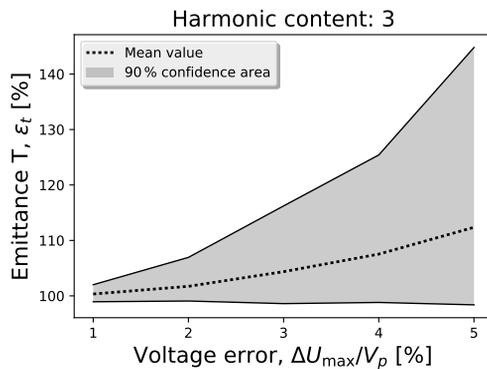
Figure 4: Simulated transverse emittance increase as a function of the voltage error.
