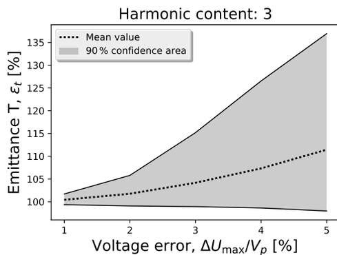
Figure 8: Predicted transverse emittance increase as a function of the voltage error.
