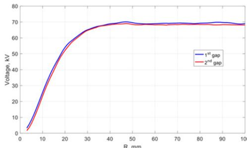
Figure 8: RF voltage along radius.
