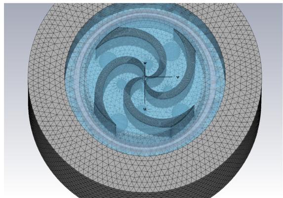
Figure 2: SC202 meshed model with mesh optimised for higher accuracy in central region.
