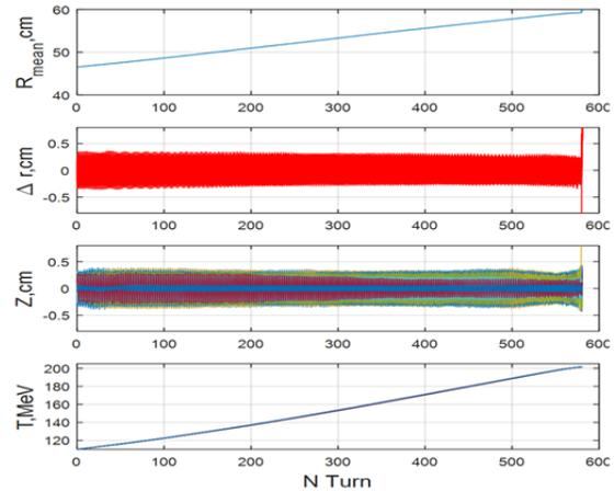
Figure 9: Particle tracking in main accelerating region until extraction in 3D electric and magnetic fields.
