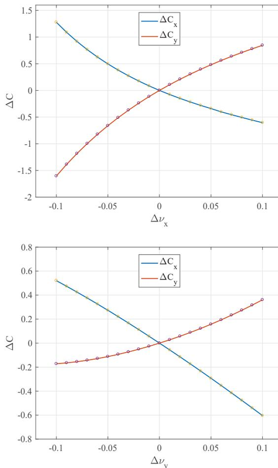
Figure 6: Chromaticity change with respect to the tune adjustment.
