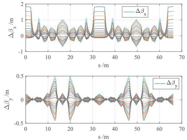
Figure 3: Beta function deviations  $\Delta\beta_x$  (upper) and  $\Delta\beta_y$  (lower) when adjusting  $\nu_x$ .
