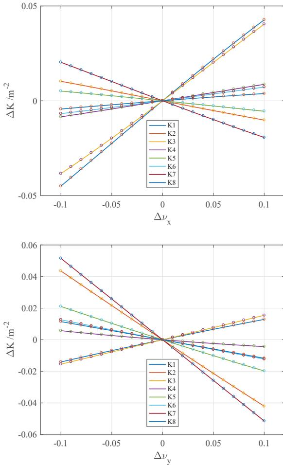
Figure 1: Quadrupole strengths adjustments with respect to the tune change (upper)  $\Delta\nu_x$  and (lower)  $\Delta\nu_y$ .
