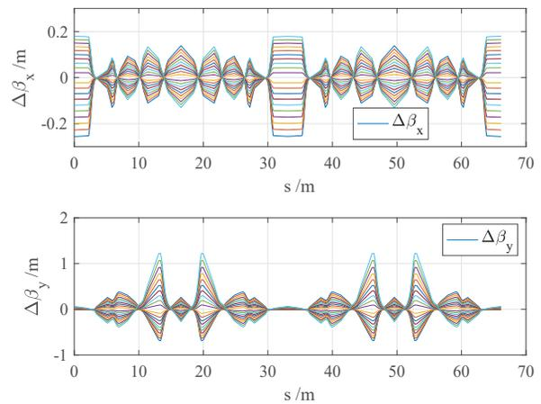
Figure 4: Beta function deviations  $\Delta\beta_x$  (upper) and  $\Delta\beta_y$  (lower) when adjusting  $\nu_y$ .
