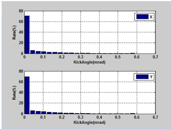
Figure 6: Corrector strength distribution. The quadrupole misalignment is 60um and BPM noise/shift error is 200/200um. The x axis is the corrector strength.
