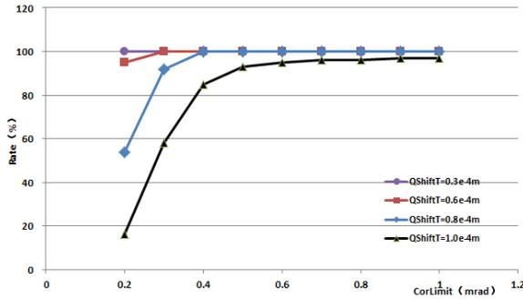
Figure 5: accumulation rate trends with different quadrupole shift in transverse. The x axis is the corrector strength limit and the y axis is the rate with 100 cases. Different colors means different quad shift in transverse and the other kinds of errors are set according to Tab. 1.
