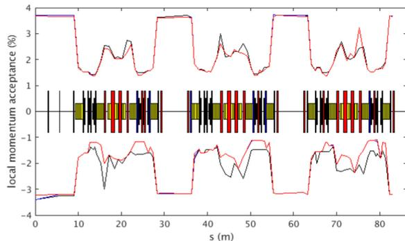
Figure 5: Local momentum acceptance along three 7BA cells of the HEPS design with high-beta straight section. In the calculation, the bare lattice is used, and RF cavity and synchrotron radiation are turned on. Three criterions determining the MA are considered, i.e., particle loss in 2000 turns (black), particle loss or crossing integer resonances (blue), particle loss or crossing integer and half resonances (red).
