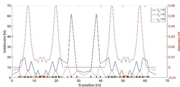
Figure 2: The opposite straight section with horizontal beta below 15 m for the convenience of installing RF cavities.
