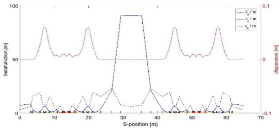
Figure 1: The straight section with horizontal beta of 90 m for the convenience of off-axis injection.
