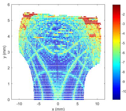
Figure 6: Effective DA at the high-beta straight section with high beta straight section (maximum  $\beta_x = 60$  m).
