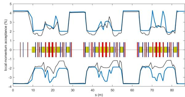
Figure 7: LMA along three 7BA cells for the HEPS design with high-beta straight section. Blue curve: LMA of the bare lattice. Black curve: Effective LMA of the bare lattice.
