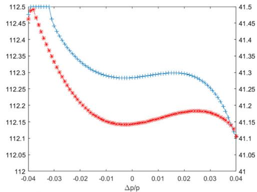
Figure 3: Effective dynamic aperture and the chromatic curves at the center of the high-beta straight section.
