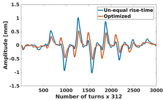
Figure 5: Perturbation measurements before (blue) and after (red) timing adjustments.
