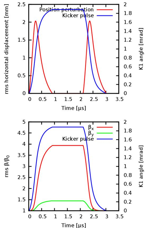
Figure 2: Injection perturbation due to the sextupole inside the injection bump.
