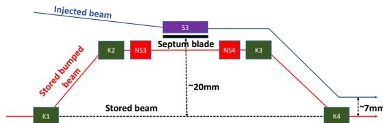
Figure 1: Schematic view of the ESRF injection.
