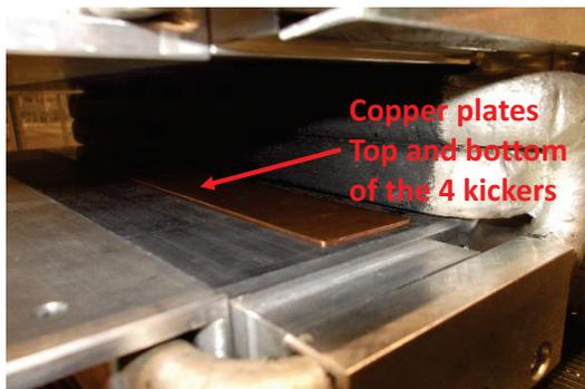
Figure 3: Field attenuation due to the copper plates and picture of the ESRF set-up.
