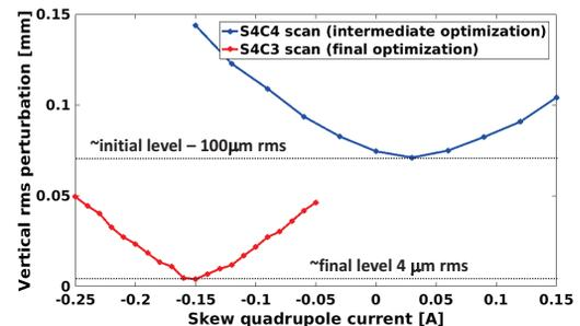
Figure 7: rms vertical orbit as a function of the skew quadrupoles current.
