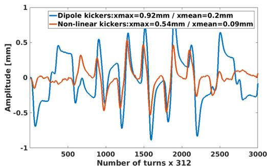
Figure 6: Perturbation measurements before (blue) and after (red) the 40 mm copper plates were installed.
