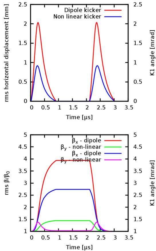
Figure 4: Injection perturbation due to the sextupole inside the injection bump with 40 mm copper plates.
