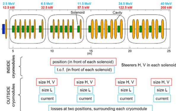
Figure 3: Beam tuning implementation for SCL.
