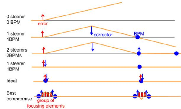
Figure 1: Transverse dipolar correction.
