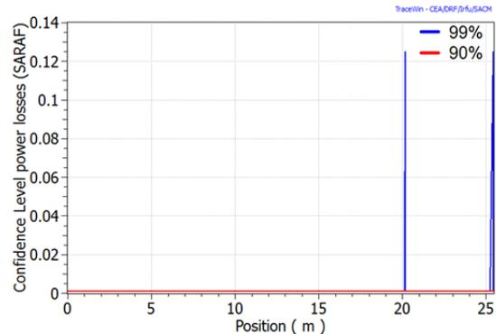
Figure 4: Beam losses along MEBT and SCL normalized to SARAF TLR (<1 is OK). Results of 1000 simulations with  $10^6$  macroparticles, in the presence of errors and correction.
