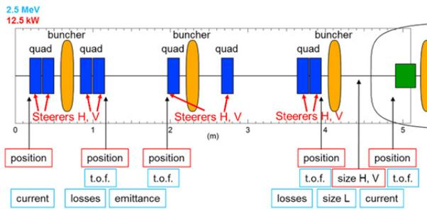
Figure 2: Beam tuning implementation for MEBT. Red, blue frames: correction, characterization measurements.
