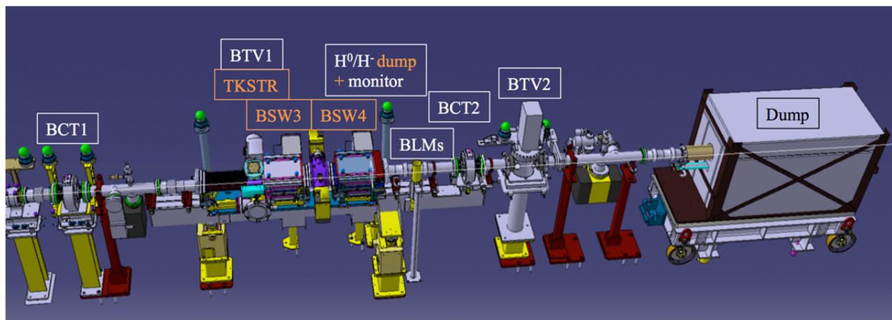
Figure 2: 3D drawing of the HST installation in the Linac4 transfer line (beam from left to right) [5].
