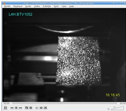
Figure 4: Online camera image of a 200  $\mu\text{g}/\text{cm}^2$  coated amorphous carbon foil installed at the HST.
