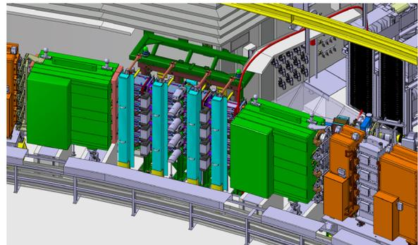
Figure 1: 3D integration drawing of the future PSB injection section, inserted between two main PSB bending magnets (green large structures) [5]. The injection line is barely visible in the middle at the right edge of the picture.
