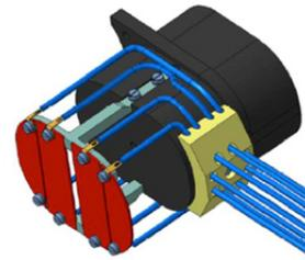
Figure 5: 3D drawing of the  $H^0/H^-$  monitor mounted on the  $H^0/H^-$  dump [8]. The two left plates will intercept the  $H^0$  beam and the right two plates the  $H^-$  beam; some basic position information is provided through the separation of the plates.
