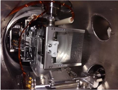
Figure 3: Stripping foil loader installed at the stripping foil test stand with a mounted foil.
