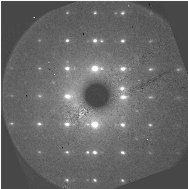
Figure 3: Present operational diffraction pattern (March 2017). Supersubstructure spots can be observed around main peaks.
