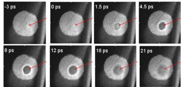
Figure 4: Electron beam image of the copper grid profile with imposed laser pump spot in it at different time.
