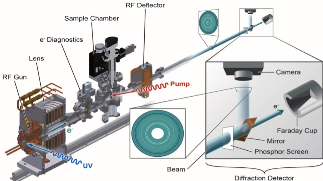
Figure 2: The layout of the initial operational configuration of the UED apparatus in Building 912 at Brookhaven National Laboratory.
