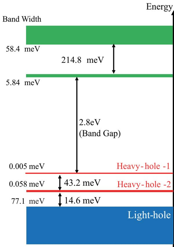
Figure 2: Energy band structure of the GaN/GaInN PC sample.
