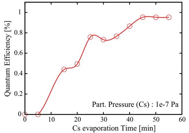
Figure 3: Quantum efficiencies as a function of Cs deposition time during the surface activation process.
