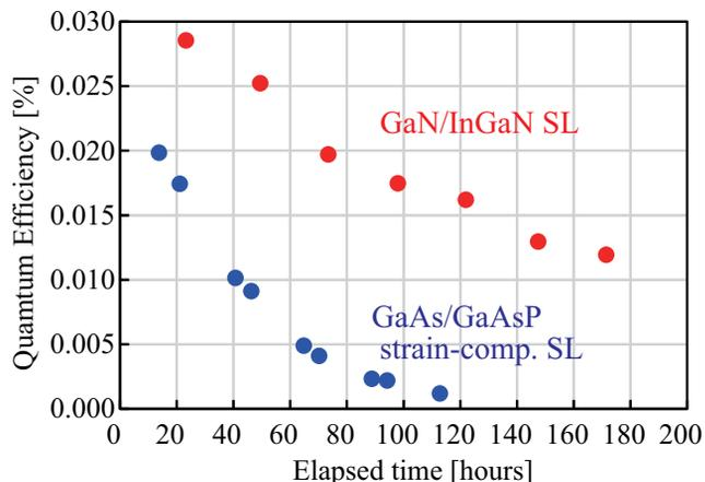
Figure 4: Quantum efficiencies as a function of the elapsed time after the activation. The result for the GaN/InGaN SL sample (red) was compared with that for the GaAs/GaAsP strain-compensated SL sample (blue).
