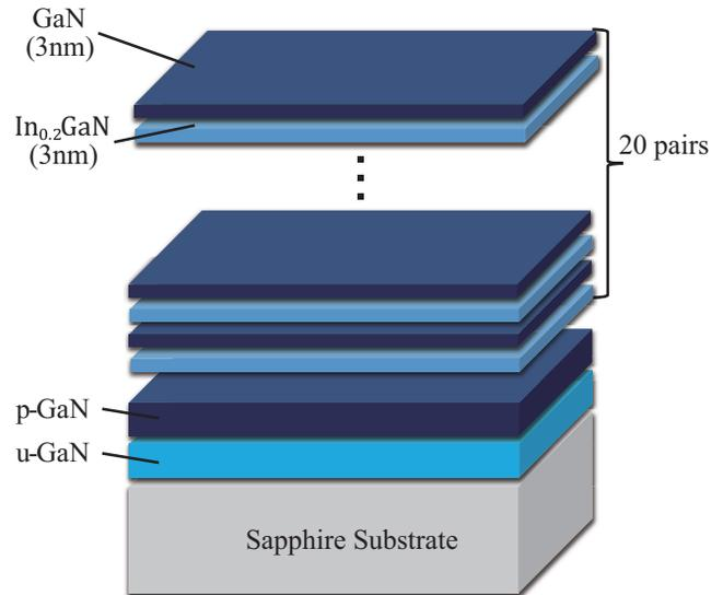
Figure 1: Schematic image of GaN/InGaN photocathode sample.
