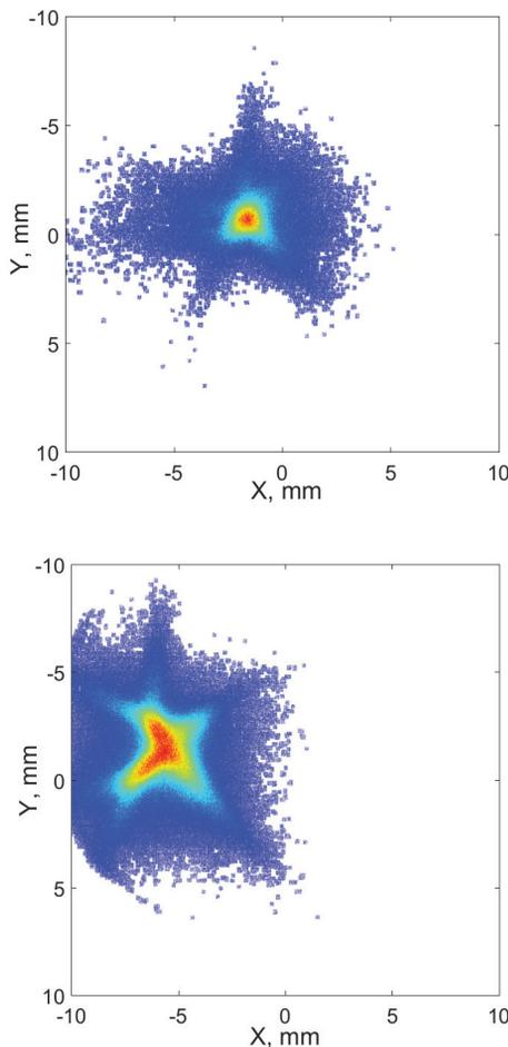
Figure 7: Transverse beam distribution recorded by the MCP for dipole currents of 0 (top) and 0.5 A (bottom). Color represents charge density in a.u.
