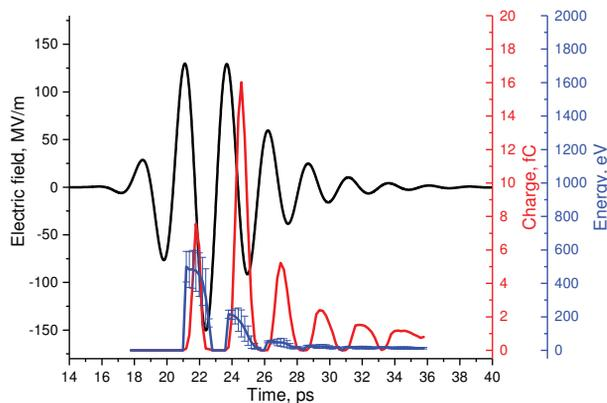
Figure 2: Beam dynamics simulations for the experimental parameters from Table 1. Each point of the red and blue curves corresponds to different times of injection of the UV pulse with respect to the THz pulse and represents beam parameters at the exit of the gun. The black curve represents the electric field amplitude at the cathode.
