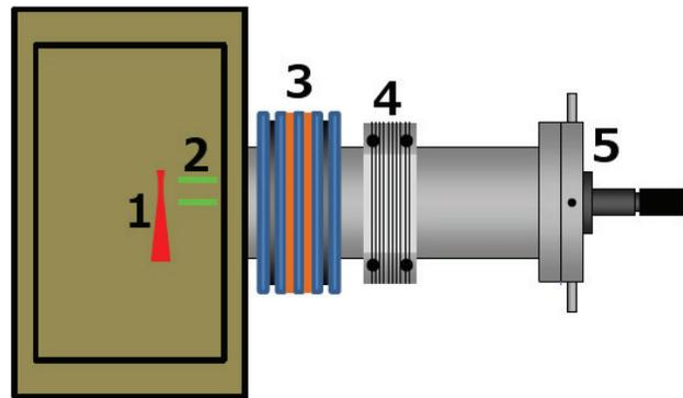
Figure 6: Experimental setup including the Horn gun (1), parallel plates (2) air coil (3), PCB steerer (4) and MCP (5).
