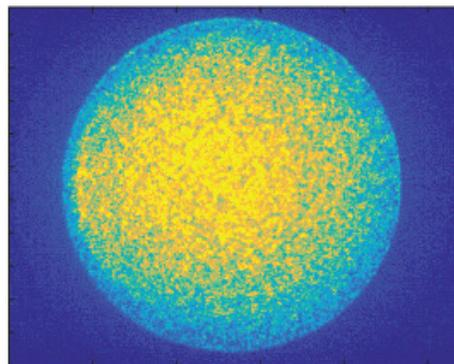
Figure 5: First example of the electron beam transverse distribution recorded using the MCP.
