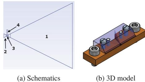
Figure 1: Schematics and 3D model of the Horn gun. Left figure numbers indicate: 1 - big horn for THz pulse coupling, 2 - small horn for THz reflection, 3 - accelerating waveguide, 4 - slit. Upper side on the right figure is made transparent for details.
