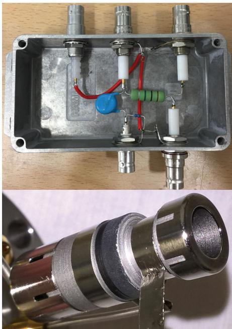
Figure 3: Channeltron (bottom) and electric circuit box (top).
