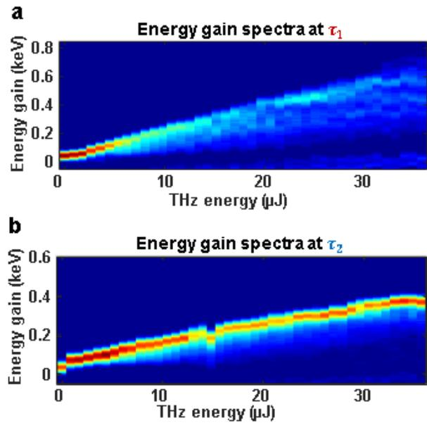
Figure 3: Accelerated electron spectra as a function of THz energy at delay (a)  $\tau_1$  and (b)  $\tau_2$ .
