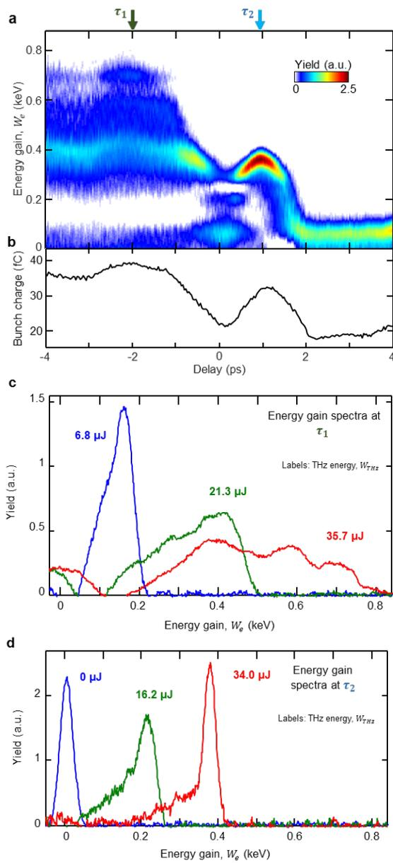
Figure 2: (a)-(b) Spectrogram showing (a) energy gain spectra and (b) bunch charge as a function of delay between UV and THz, at max THz energy. (c)-(d) Accelerated electron spectra at delay (c)  $\tau_1$  and (d)  $\tau_2$  for several THz energies.
