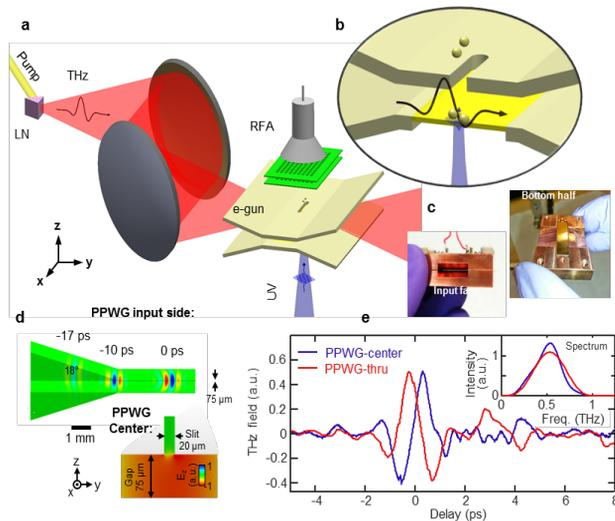
Figure 1: (a) Schematic of UV-triggered THz gun. (b) Photoemission method for electron injection. (c) Photos of the fabricated THz gun and (d) snap-shots of the simulated field profile within the proposed THz gun. (e) Temporal signature of the THz pulse used for electron acceleration.
