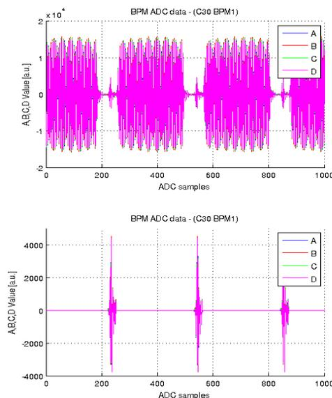
Figure 2: ADC sampled data without gate (top) and with gate (bottom).
