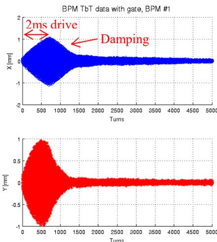
Figure 4: Gated BPM TbT data with bunches in the gap excited to ~1mm peak. The duration of excitation is 2ms.
