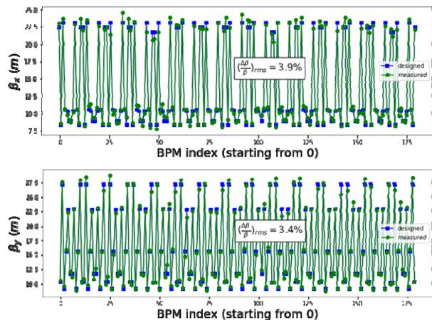
Figure 5: Beta-function measured from gated BPM TbT data. X/Y beta-beat was ~3.9%/3.4%.
