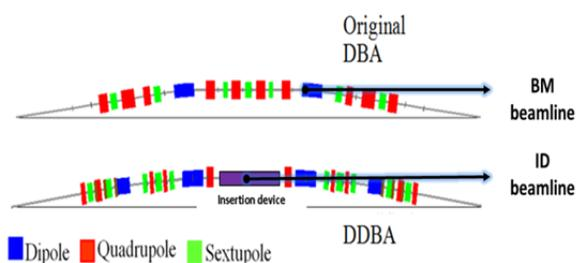
Figure 1: Schematic diagram of the existing DBA cell and the modified DDBA cell.
