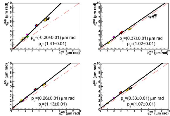
Figure 2: Emittance from BGI vs wire scanners. The figure has to be redone with the latest values of the measured betas
