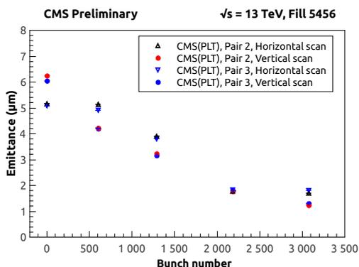
Figure 4: Off-line  $\epsilon_{H,V}$  measured from the emittance scan analysis by CMS using the PLT data.
