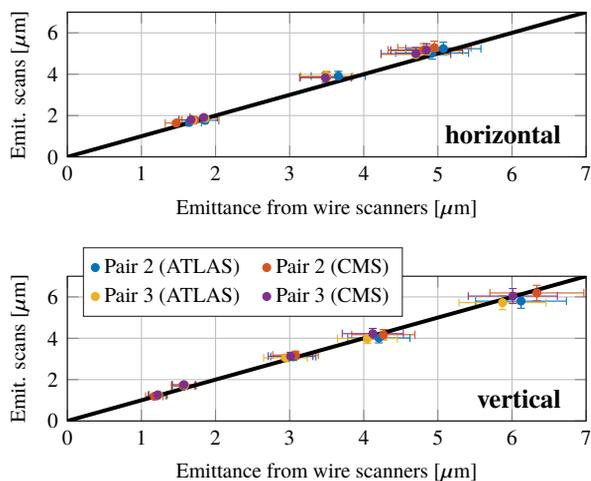
Figure 3:  $\epsilon_{H,V}$  from the emittance scan analysis compared to the WS measurements. The diagonal is unity.
