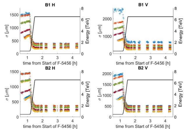
Figure 1:  $\sigma_{H,V}$  evolution, bunch-by-bunch, as measured by the WS. The adiabatic shrinking of the beam size during the energy ramp is observed.
