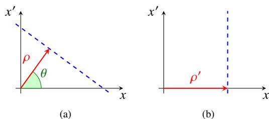
Figure 4: Correspondence between a phase-space profile integral line (dashed line) at the reconstruction location (a) and at the measurement location (b). The red arrows identify the distance of the integral line from the origin of the axes at the two locations.
