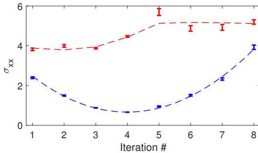
Figure 1: Horizontal beam variance  $\sigma_{xx}$  measured at the screen for different settings of quadrupole settings. Dashed are the expected values from the fitted Twiss parameters.
