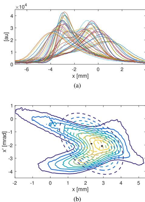
Figure 5: Measured horizontal beam profiles (a) used for the transverse phase-space tomographic reconstruction in (b). Dashed is the phase-space reconstruction using the simpler quadrupole scan technique.
