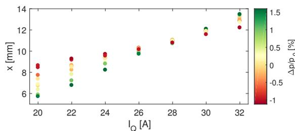
Figure 3: Horizontal beam position  $x$  measured at a screen as a function of quadrupole current  $I_Q$ . The colour code is the beam energy variation with respect to nominal.
