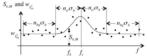
Figure 3: Estimation of background noise and beam intensity.
