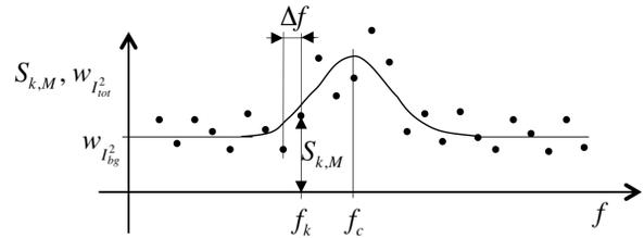
Figure 1: Spectral power density as a superposition of the Schottky signal from the beam and background noise.
