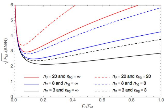
Figure 4: Statistical error of Schottky based Intensity Measurement.
