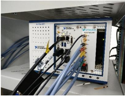
Figure 2: data acquisition board and PXIe chassis for BTB on-line measurement.
