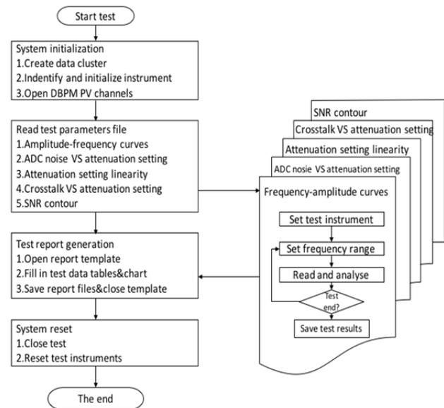
Figure 4: Algorithm flow pattern of test system.
