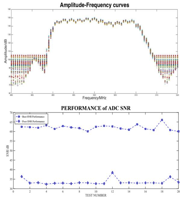
Figure 7: amplitude-frequency curves and SNR performance of 20 sets DBPM processor.
