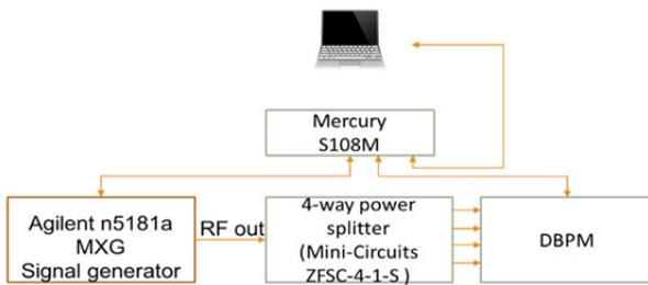
Figure 2: Hardware architecture.
