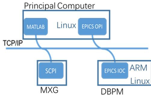
Figure 1: The overview architecture of the test system.
