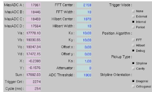
Figure 3: digital beam position processor EDM panel.
