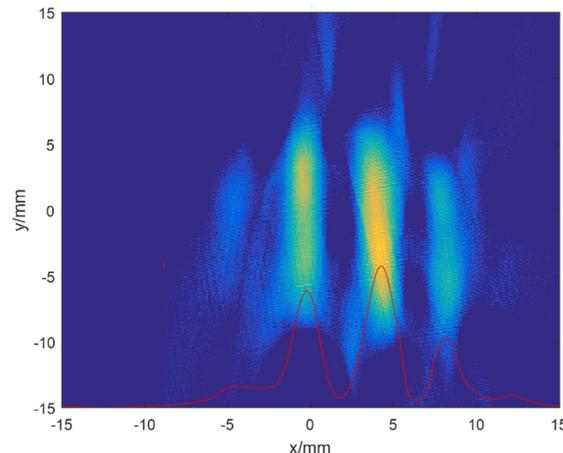
Figure 8: Reconstructed profile with ART algorithm from 33 projection with the mask inserted.
