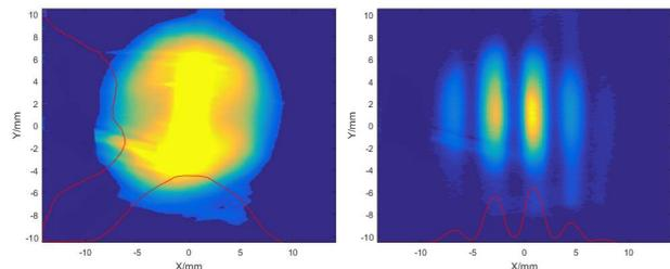
Figure 5: Beam profile monitored by scintillator screen. left: w/o mask, right: with mask inserted.
