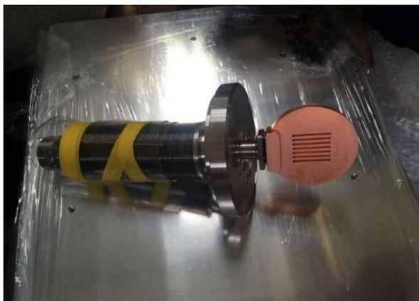
Figure 6: Mask made of copper.
