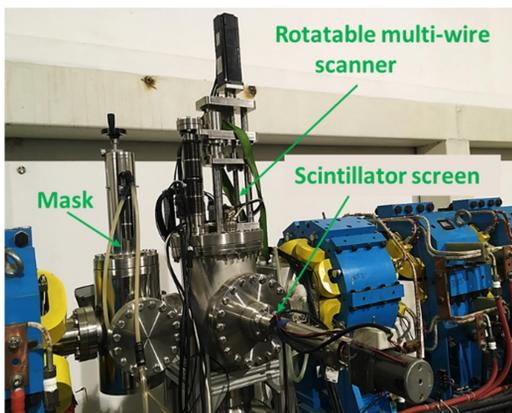
Figure 3: Experimental set-up.
