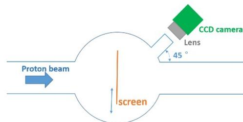
Figure 1: Schematic diagram of profile monitor based on scintillator screen.
