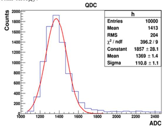
Figure 4: Test energy spectrum of  $\text{Bi}^{207}$ .
