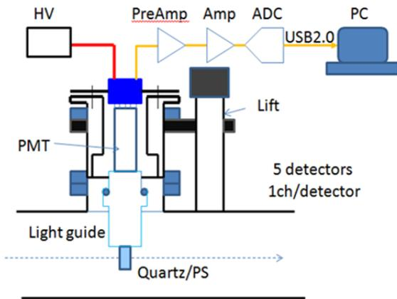
Figure 3: The schematic of weak current monitors.
