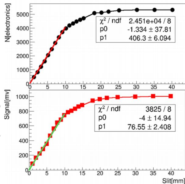
Figure 7: Electron number on detector 3 with the slit 5 changes.
