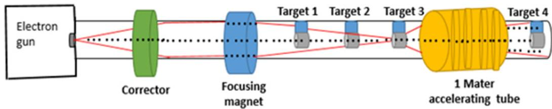
Figure 5: Schematic diagram of actual beam photometry.
