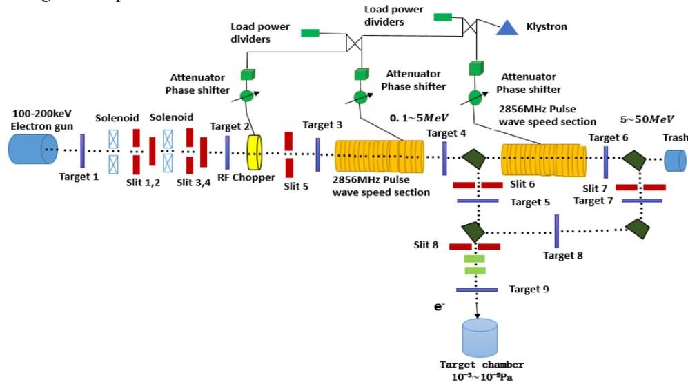
Figure 1: Accelerator device layout.
