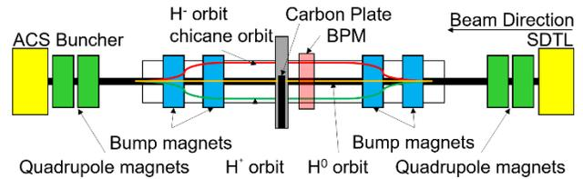
Figure 1: Device Location in MEBT2 Diagnostics Line.
