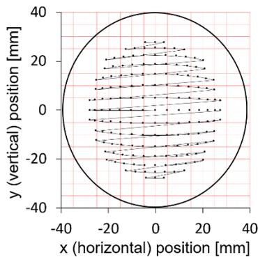
Figure 6: Mapping of the BPM position characteristics moving the thin wire.
