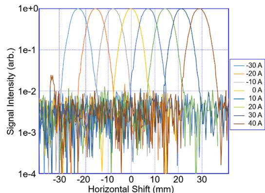
Figure 7: Beam profile measurement results with several current-sets.
