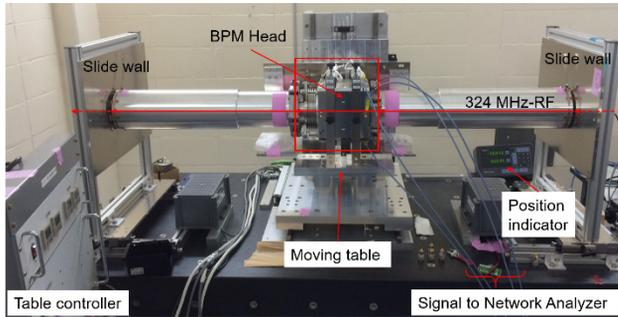
Figure 5: Overview of calibration bench for BPM.
