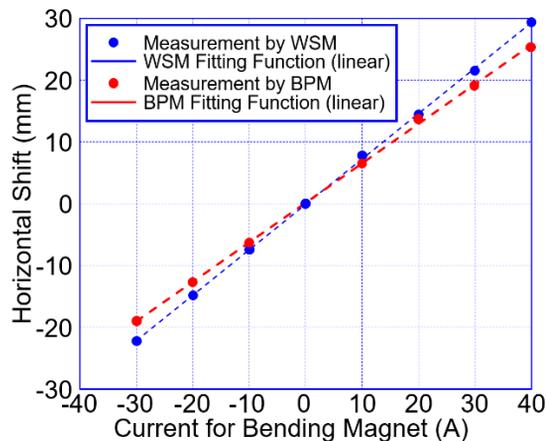
Figure 8: Beam position indication by BPM and WSM.
