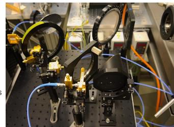
Figure 1: The incoming synchrotron radiation is first polarized and then divided into four beams by 3 wire-grid beam splitters. The split beams are focused onto four detectors, each one sensitive at different frequency range. The single shot measurements are sampled and read out by the *KAPTURE* system.
