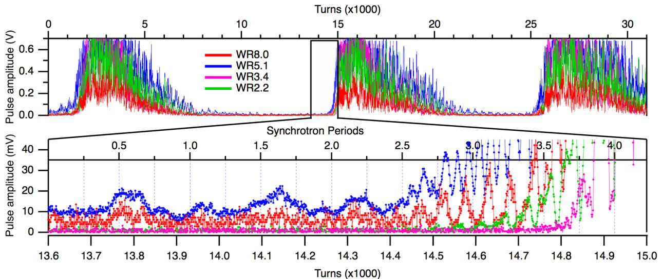
Figure 4: Measured turn-by-turn amplitudes of the four different diodes (1000 turns  $\approx$  0.368 ms  $\approx$  3 synchrotron periods). The bottom panel shows a zoom-in to the beginning of a burst. Every point is a measured pulse amplitude, the line is to guide the eye.
