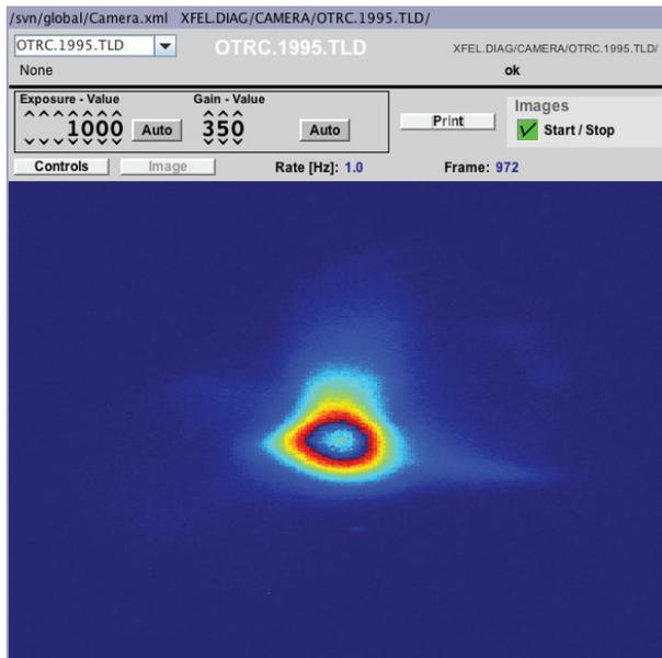
Figure 4: Display of the transverse beam distribution with a screen station at 1995 m behind the electron source during the first beam commissioning.
