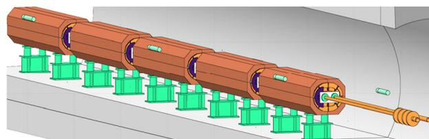
Figure 3: First approach to post-LS2 layout of cell 5 in LHC's IR7.
