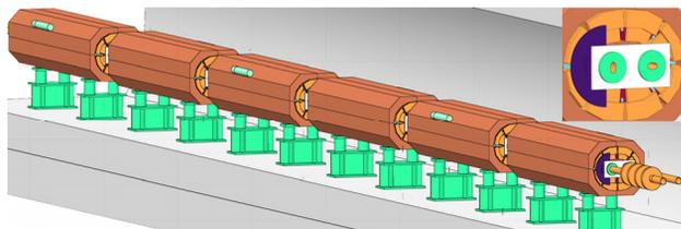
Figure 2: Present layout of the Q5 magnet, with 6 MQW module and a TCAPC passive absorber for the protection of incoming B1 losses.
