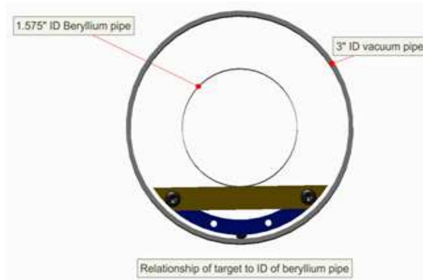
Target is installed 2.05 m from the IP in the Yellow ring
