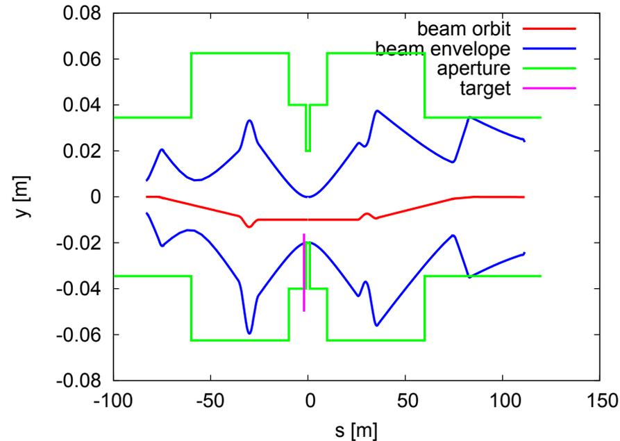
At  $\beta^* = 8$  m, a 10 mm vertical orbit bump allows the target to become the limiting aperture at **16 mm** from the beam pipe center
