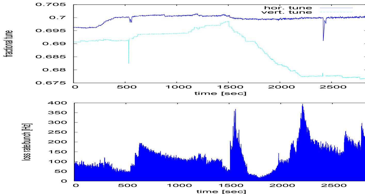
Loss rates during the tune scan with fixed collimator position at 11.5 mm
