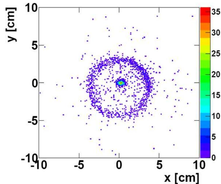
Large number of background collision events on detector beampipe
