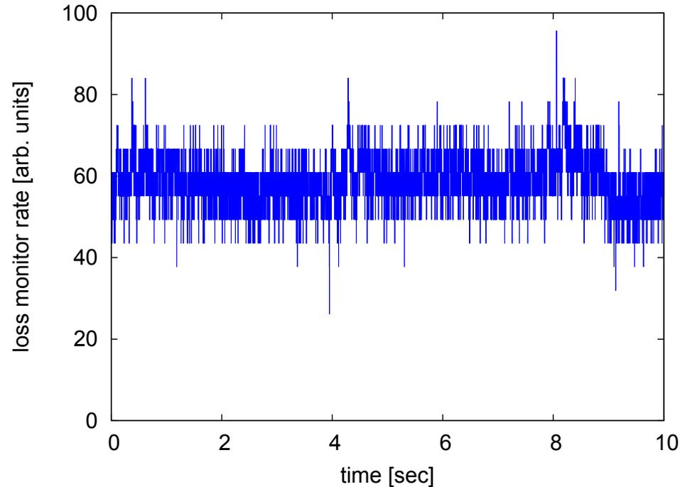
No fast rate fluctuations due to orbit jitter or target vibration
