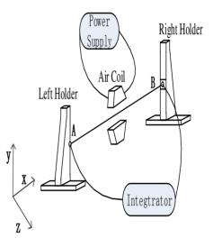
Figure 1: Schematic of the stretched wire system.
