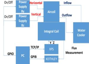
Figure 3: Functional diagram of air coil magnetic field measurement test setup.
