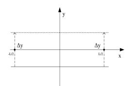
Figure 2: Parallel movement for the measurement of the first field integral.
