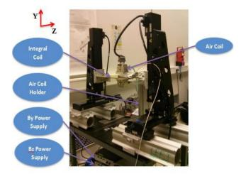
Figure 4: View of the mowing wire setup designed for air coil measurements.
