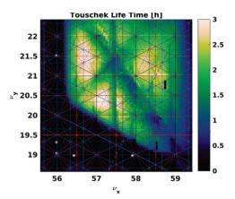
Figure 3: C2 tune-scan with respect to lifetime;  $\epsilon_y = 5 \text{ pm}$ , i.e. coupling=4%.
