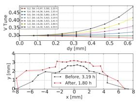
Figure 2: Top: C2 linear optics optimisation example: vertical detuning with vertical amplitude, DA and lifetime, for  $\alpha_y$  varying from 0.2 to 1.2 (initial  $\alpha_y = 0.7$ , cyan line). Bottom: DA and lifetime comparison of C2, before and after optimisation (black and red lines respectively).
