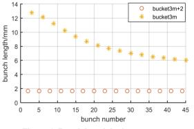
Figure 4: Bunch length in the new pattern.
