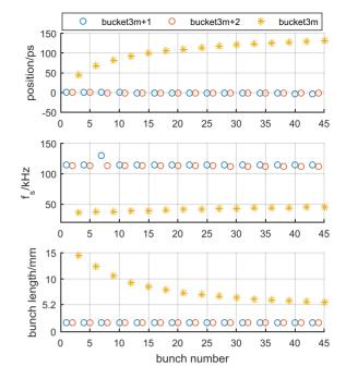
Figure 3: Synchrotron phase position (top), synchrotron frequency (center), and bunch length (bottom).
