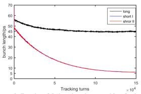
Figure 2: Results of 3 damping times tracking for length variation. Long, short I and short II bunches length variation are indicated in black, blue, red. The blue line coincides with the red one approximately. The final bunch length after 3 damping times are 45ps, 6ps and 6ps.
