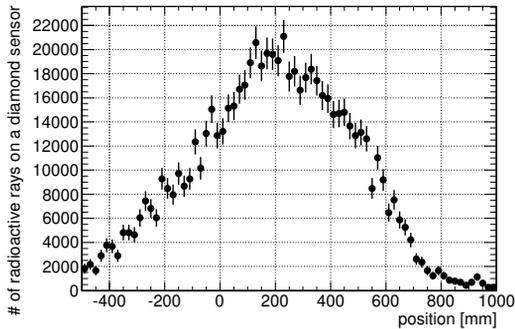
Figure 11: The number of radioactive rays observed on a diamond detector as a function of the position where it is placed.
