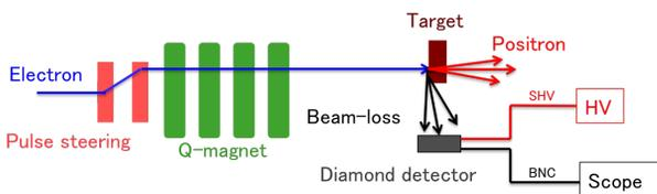
Figure 6: Schematic of the system used for the beam tests at the SuperKEKB LINAC.
