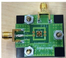
Figure 5: Installed diamond detector with a dedicated PCB.
