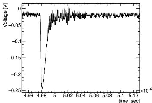
Figure 7: Typical waveform of the signal induced in the diamond detector.
