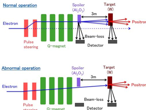
Figure 3: Schematic of positron production system in the normal (top) and abnormal (bottom) operation.
