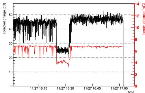
Figure 9: Collected charges in the diamond as a function of time.
