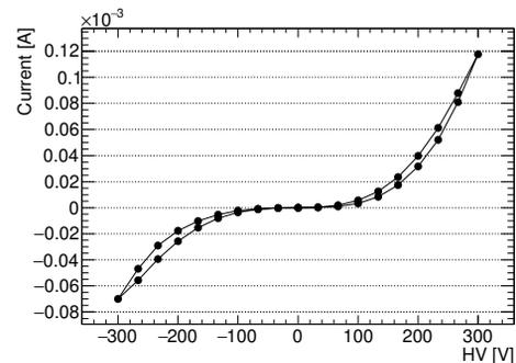
Figure 4: Leakage current as a function of bias voltage.
