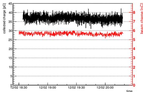
Figure 8: Collected charges in the diamond as a function of time.
