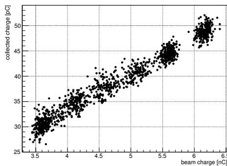
Figure 10: Relation between the induced signal in the diamond detector and electron-beam charges.
