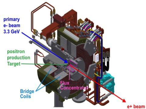
Figure 1: Positron production system at the SuperKEKB LINAC.
