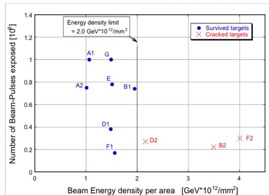
Figure 2: Target damage threshold as a function of beam energy density and the number of beam-pulses exposed [2].
