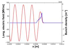
(b) Lineout along x-axis of bunch density (blue) and longitudinal electric field (red).
