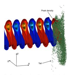
Figure 7: Isosurface plot of longitudinal electric field and bunch macroparticles for 3D simulation of a realistic CLARA-FE bunch. The isosurfaces are clipped in the x-y plane for visibility. The longitudinal coordinate is x.
