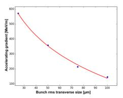
Figure 5: Dependence of average accelerating gradient for particles in the tail of the bunch on bunch radius, for a plasma density of  $3\times10^{22}$  m<sup>-3</sup>. The red line shows a least-squares fit to log(const./ $\sigma_r$ ), the expected relation from the linear theory for a cigar-shaped bunch [8]
