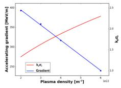
Figure 4: Dependence of average accelerating gradient for particles in the tail of the bunch on plasma density, for a bunch radius of 50  $\mu$ m. The variation of the product  $k_p\sigma_z$  is also shown, and the gradient plot includes a least-squares fit to a linear function.
