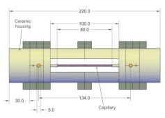
Figure 1: Initial design of a plasma discharge cell for PWFA experiments with CLARA-FE. Dimensions are in mm.
