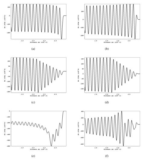
Figure 2: a,b) Single bunch of 8 nC, c,d) eight bunches with 1 nC each and separated by  $\lambda_p$ , e,f) eight bunches with 1 nC each and separated by  $\lambda_p/2$  at the first time step and after 100 mm propagation into the plasma, respectively.
