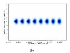
Figure 1: a) Arrangement of eight bunches with separation of  $\lambda_p$ , b) same bunches after 100 mm propagation into the plasma.
