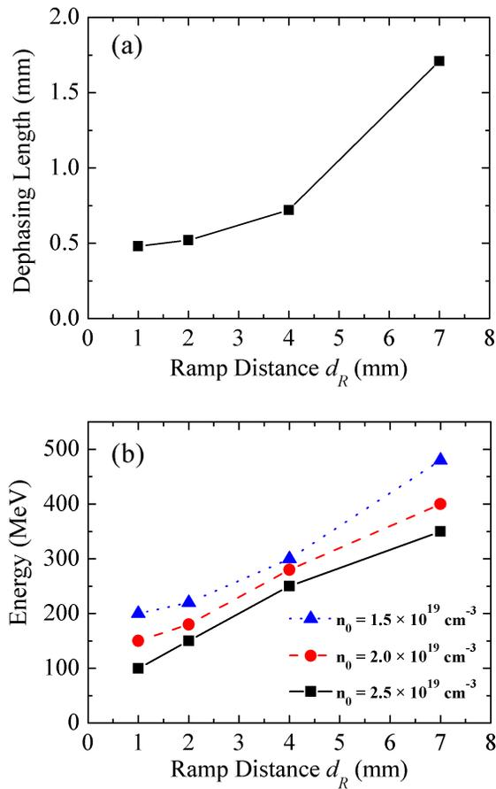
Figure 4: (a) The dephasing length depending on the ramp distance  $d_R$  (b) PIC simulation results with peak energy as a function of ramp distance for  $n_0 = 1.5 \times 10^{19} \text{ cm}^{-3}$ ,  $n_0 = 2 \times 10^{19} \text{ cm}^{-3}$ , and  $n_0 = 2.5 \times 10^{19} \text{ cm}^{-3}$ .
